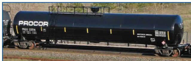
TC/DOT 112J340W 33,800 USG tank car in anhydrous ammonia service
